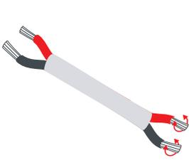
1. Cut a length of connection wire to run from Receiver to Tape Light location. Strip 1/4" insulation from both ends of wire, and fold stripped wires in half.
